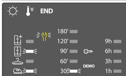
The presence of wrench symbol signals a malfunction. Carry out the operations described. Switch the dryer off and unplug it. Open the door immediately and pull laundry out, to allow the heat to dissipate. Wait for about one hour. Reconnect the dryer to the power supply, load the laundry and restart the drying cycle.
