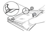
**4.** Refit the upper edge: A click will indicate correct positioning. Make sure the seal is secure before refitting the door.
