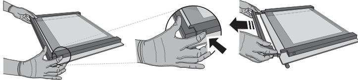
2. Lift and firmly hold the inner glass with both hands, remove it and place it on a soft surface before cleaning it.
