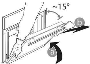
2. Close the door as much as you can. Take a firm hold of the door with both hands – do not hold it by the handle. Simply remove the door by continuing to close it while pulling it upwards at the same time until it is
