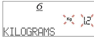
To set the function correctly, follow the indications on the display, when prompted, and turn the **adjustment knob** to set the required value then press  $\checkmark$  to confirm.
