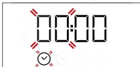
Use + or - to set the hour and press to confirm. The two digits for the minutes will start flashing. Use + or - to set the minutes and press to confirm. Please note: When the icon is flashing, for example following lengthy power outages, you will need to reset the time.
