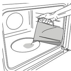
To start the Steam function, pour 200 ml of drinking water in the oven bottom. Select the function turning clockwise the selection knob on the relevant icon, and the thermostat knob in any position between 160 and 180°C (as suggested by the icon). The function will start and the display will show the current time of the day. No preheating is needed. To end the cooking, turn the selection knob on **0** position. During Steam cooking do not open the door and never top up the water.
