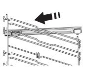
Remove the shelf guides from the oven and remove the protective plastic from the sliding runners.
