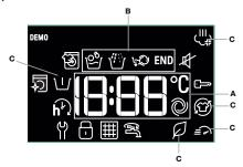
The duration of the available wash cycles and the remaining time of a running cycle appear in section A (the display will show the maximum duration of the cycle chosen, which may decrease after several minutes, since the effective duration of the programme varies depending on the wash load and the settings chosen); if the DELAYED START option has been set, the countdown to the start of the selected wash cycle will appear.
