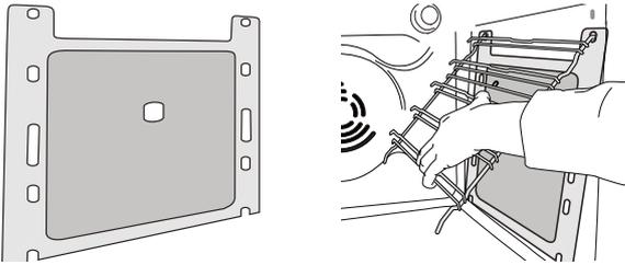
To make best use of the catalytic panels' self-cleaning properties, we recommend heating the oven to 200 °C for around one hour using the “Convection Bake” function. The oven must be empty during this time. Then leave the appliance to cool down before removing any remaining food residues using a nonabrasive sponge.
