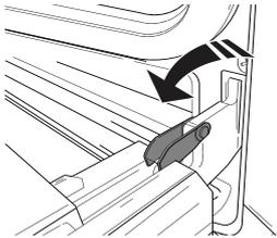
**2.** Close the door as much as you can. Take a firm hold of the door with both hands – do not hold it by the handle. Simply remove the door by continuing to close it while pulling it upwards (a) at the same time until it is released from its seating (b).
