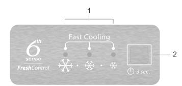
1. Indicator Leds (to display the current temperature setpoint or the Fast Cooling function) 2. On/Stand-By Button / **Temperature Button**
