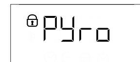
Once the cycle has been completed, the door remains locked until the temperature inside the oven has returned to a safe level. Air the room during and after running the Pyro cycle.
