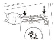
**3.** To reposition the heating element, lift it up, pulling it slightly towards you, making sure it comes to rest on the lateral supports.
