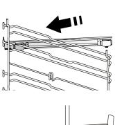
Remove the shelf guides from the oven and remove the protective plastic from the sliding runners.
