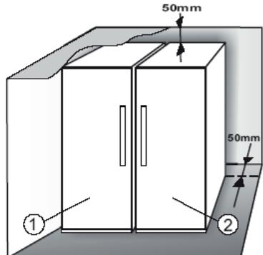
We recommended installing two appliances together using the linking-kit ③ (as shown on the drawing). You can buy it in Service.
