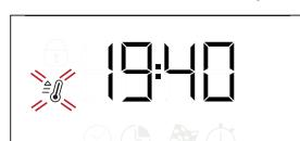
Please note: During cooking you can change the function by turning the *selection knob* or adjust the temperature by turning the *thermostat knob*. The function will not start if the *thermostat knob* will be on **0**. You can set the cooking time, cooking end time (only if you set a cooking time) and a timer.
