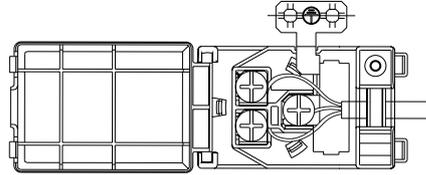
**The appliance must be connected to the electricity supply by means of an all-pole disconnect switch with minimum contact gap of 3 mm.**
