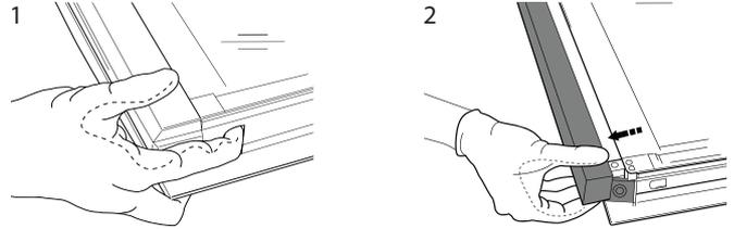
Lift and firmly hold the inner glass with both hands, remove it and place it on a soft surface before cleaning it (3).
