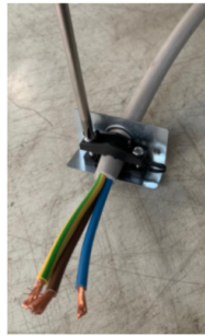
Fix power cord to the plastic holder.
