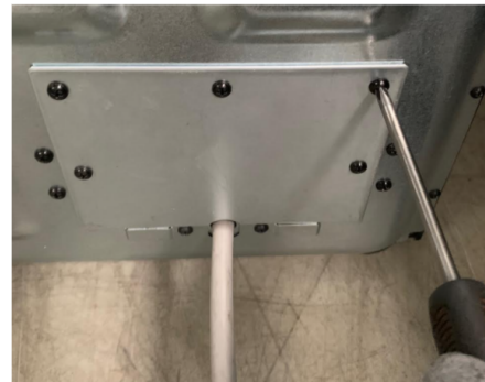
Assemble cover and tighten screws.
