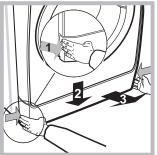
2. Loosen the drainage pump cover by turning it anticlockwise: it is normal for some water to leak out;
