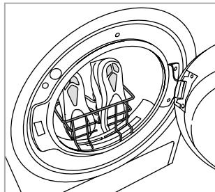
Remove the door filter and place the shoe rack. Put shoelaces into the shoes with the shoe tips facing downwards and the soles frontwards. **Do not add garments or other shoes into the drum.** Position the door filter back in place at the end of drying.
