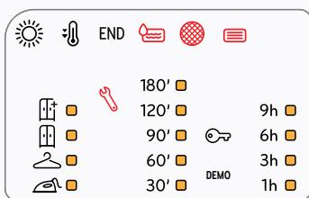
The presence of wrench symbol signals a malfunction. Carry out the operations described. Switch the dryer off and unplug it. Open the door immediately and pull laundry out, to allow the heat to dissipate. Wait for about one hour. Reconnect the dryer to the power supply, load the laundry and restart the drying cycle.
