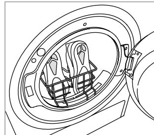
Remove the door filter and place the shoe rack. Put shoelaces into the shoes with the shoe tips facing downwards and the soles frontwards. **Do not add garments or other shoes into the drum.** Position the door filter back in place at the end of drying.
