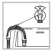
alternatively, rest it on the side of a washbasin or bathtub, fastening the duct supplied to the tap (see figure). The free end of the hose should not be underwater.
