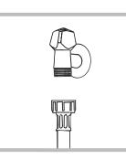
1. Connect the supply pipe by screwing it to a cold water tap using a <sup>3</sup>/<sub>4</sub> gas threaded connection (*see figure*). Before performing the connection, allow the water to run freely until it is perfectly clear.
