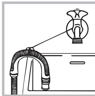
Alternatively, place the drain hose over the edge of a washbasin or bathtub, by fastening the guide (which can be purchased at the technical assistance centre) to the tap (see figure). The free end of the hose
