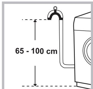
Connect the drain hose, without bending it, to a drainage duct or a wall drain located at a height between 65 and 100 cm from the floor.
