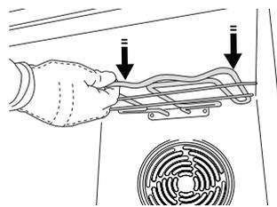
**2.** To return the heating element to its position, lift it up, pull it slightly towards you and make sure that the tab support is in its proper seating.
