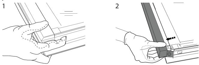
visible in the left-hand corner and the clear surface (not printed) is facing up. First insert the long side of the glass indicated by "R" into the support seats, then lower it into position (4). Refit the upper edge (5): a click will indicate correct positioning. Make sure the seal is secure before refitting the door.
