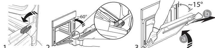
Put the door to one side, resting it on a soft surface. Refit the door by moving it towards the oven, aligning the hooks of the hinges with their seating and securing the upper part onto its seating.
