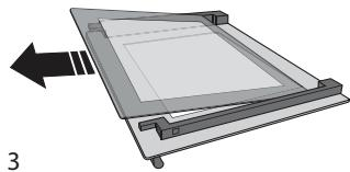
To correctly reposition the inner glass, make sure that the "R" is
