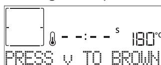
When the display shows the relevant message, if required press  to start a five-minute browning cycle. You can stop the function at any time by pressing  to switch the oven off.
