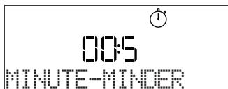
An audible signal will sound and the display will indicate once the minuteminder has finished counting down the selected time.
