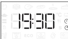
Please note: Programming a delayed cooking start time will disable the oven preheating phase: The oven will reach the temperature you require gradually, meaning that cooking times will be slightly longer than those listed in the cooking table.
