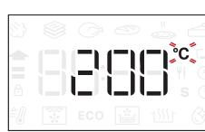
When the °C icon flashes on the display, turn the knob to change the value, then press to confirm and continue to alter the settings that follow (if possible).
